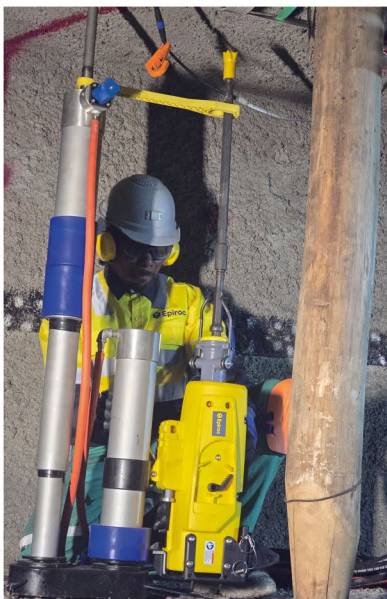
RD100RB Hydraulic rock drill mounted on the multi-stage support drilling leg
