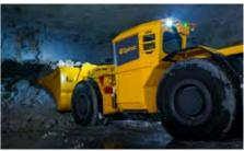
With its integrated load weighing system, the Scooptram ST7 provides operators instant feedback on productivity and makes it easy to plan tonnage output over time.
