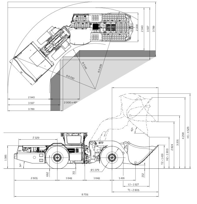
All dimensions are shown in millimeters (mm). Dimensions and calculations shown are based on standard vehicle configuration with 27 mm tire deflection, unloaded.
