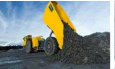
The robust dump box has a load capacity of 54 metric tonnes and the load-weighting system monitors the loading process.
