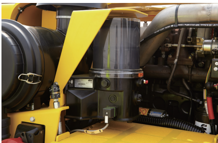
The Scooptram ST4's automatic lubrication system ensures consistent greasing of key components, reducing service intervals and maximizing uptime in demanding underground environments.
