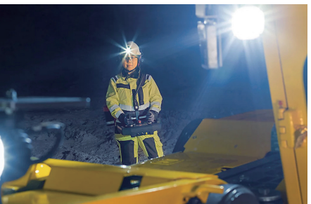
Radio Remote Control (RRC) for line-of-sight operations, offers an effective way of working inside stopes and areas exposed to risks of falling rock. When personal safety cannot be guaranteed, RRC enables an operation to take place from a safe distance.
