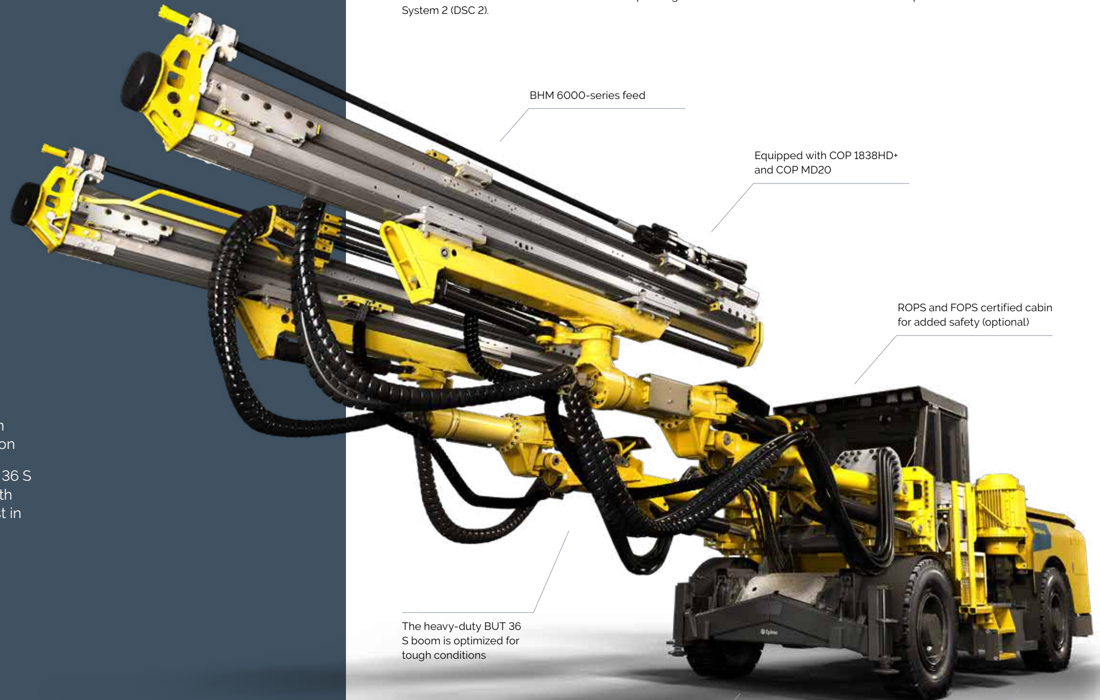
Equipped with optional BUT 29 HD booms, Boomer M2D becomes well-suited for operating in smaller drift sizes.
