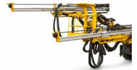
The lighter BUT 29 HD booms allow for a service platform to be added on the machine (optional).
