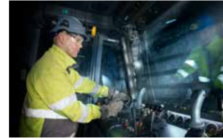
The operator panel has adjustable height, and a good and productive working environment with the Direct Control System 2 (DSC 2).
