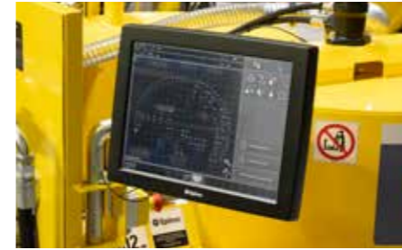
All operations of the Unigrout M10 S is controlled from an easily accessible touch screen.
