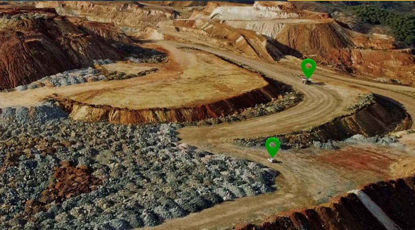
Blast support is a digital decision support tool to ensure improved personnel safety at blasting. 3D visualization with open space positioning gives the control room an overview of everyone's location.
