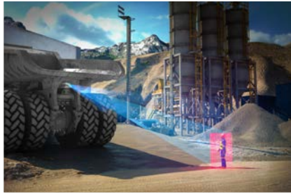
Epiroc offers the highest Collision Avoidance Level for safer mining operations: Level 9. If the operator does not act, the system will take interventional control and stop the machine.
