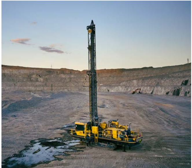
In October, Epiroc announced a large order for surface mining equipment in Australia from Newmont Corp., one of the world's leading gold producers. The rigs, among others the Pit Viper 231 rotary blasthole drill, will be operated tele-remotely, i.e. run with automation.
