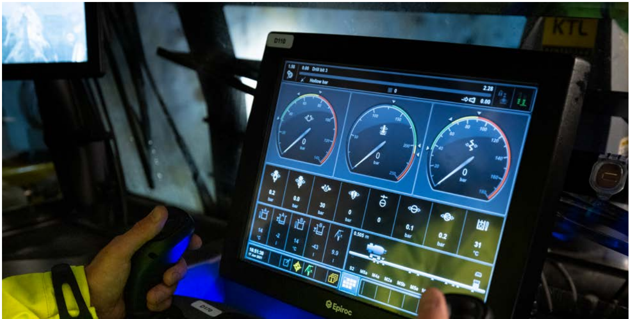
The Boltec rock bolting rigs M10 S and E10 S are designed to give increased productivity and bolt installation quality thanks to intelligent options and compatibility with different bolt types. Thanks to a new operator control panel, reduced noise levels and better visibility, operator ergonomics are also improved. The battery-electric versions are indicated with SG in the model name, which stands for Smart and Green - Boltec M10 SG and Boltec E10 SG.
