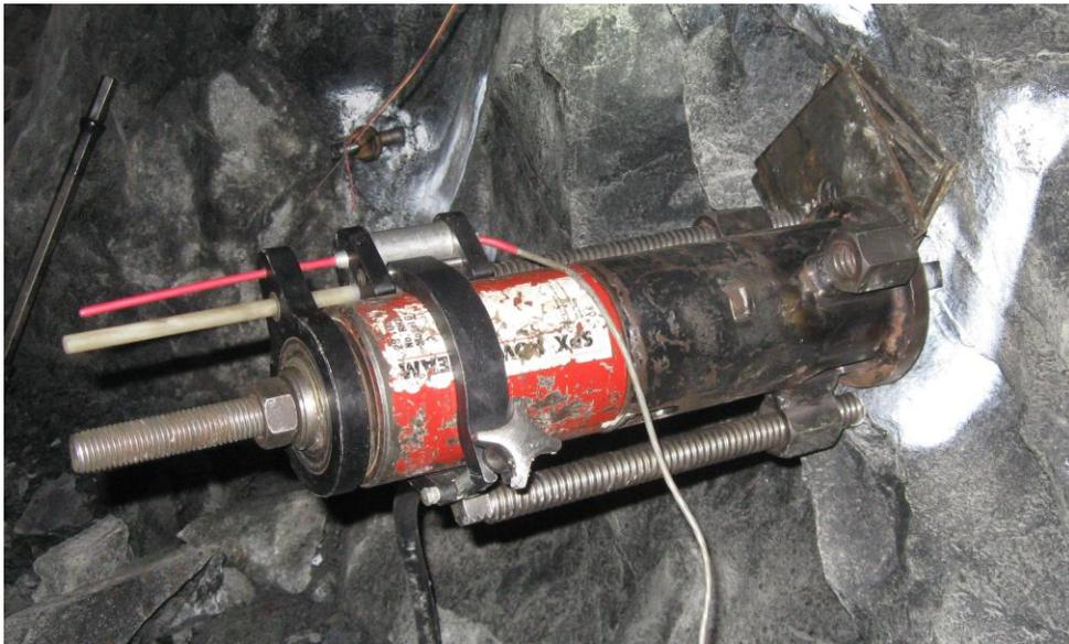
**Figure 1.** The pull test unit being used at Kidd Mine (courtesy of Jenmar Canada)
